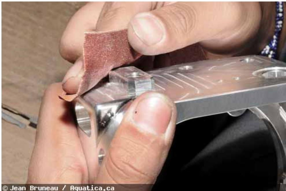
After manual deburring there are still some external sharp edges that need to be addressed, and so the shell will be put in a tumbler. The tumbler is a donut shaped machine loaded with pellets of different sizes. In the machine, the shell will be subjected to a lengthy period of vibration, which will cause the pellets to rub against it and dull out all sharp edges. This machine is horrendously noisy and any conversation between people is put to a standstill during this process.
