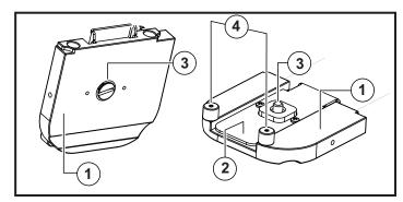
3. The power switch must be in the same position on both the housing (# 43) and on the camera body.
