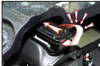
7. If using a Monitor, confirm the connection and secure all wiring and cable that could potentially get caught in between the rear and front of the housing, this is a critical and essential thing to check.
