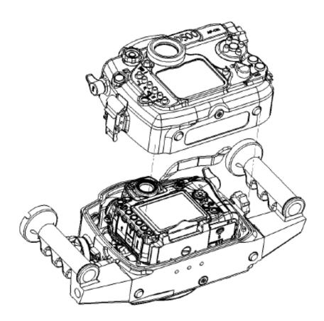
[IMPORTANT] In the event that you feel any unusual resistance when attempting to close the rear door, do not force the closure. Reopen, inspect carefully for any potential obstruction such as *ON/OFF* switch position and try again.
