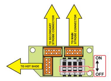
Note that none of the offered flash triggering options on the AD500 NOTE: housing are TTL compatible.
