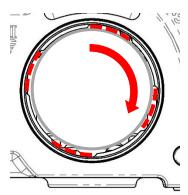
Push with even force on both sides of the port or extension ring until you feel it snap into place. Make sure the bayonet is completely inside the housing.
