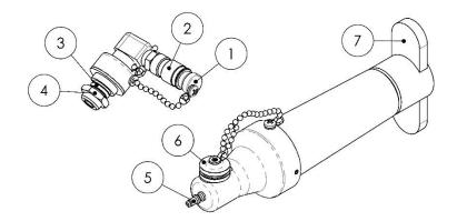
STEP 3: Remove the valve plug (#1) by sliding the quick-disconnect collar (#2).
