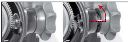
PULL AND ROTATE CLOCKWISE THE RELEASE DISK TO DISENGAGE THE FOCUS KNOB PINION GEAR OF THE EXTENSION.
