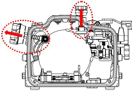
**STEP 8:** Slide the saddle and camera inside the housing using the two guiding pins. Push it all the way through until you hear the locking mechanism click in the housing. Perform a check by pulling on the saddle to ensure it is firmly attached to the housing.
