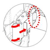
**STEP 2:** Rotate both latches to free them from the front hooks and pull out the rear portion.
