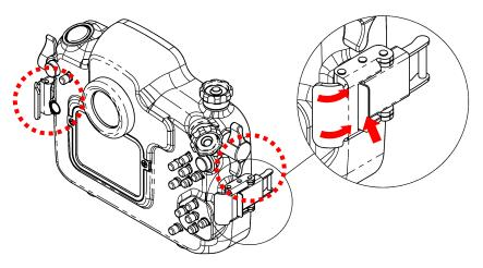
**STEP 5:** Pull the latches out so they don't interfere with the front portion hooks upon closing.
