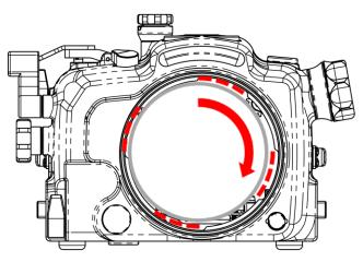
**STEP 4:** Push with even force on both sides of the port or extension ring until you feel it snap into place. Make sure the bayonet is completely inside the housing.
