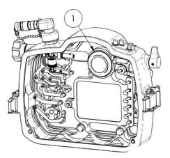
STEP 2: Carefully pull the eyepiece body out of the housing.
