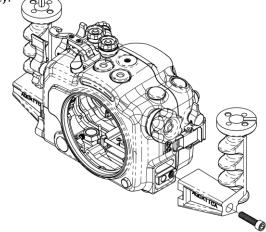
STEP 2: If you are adding any shoes, brackets or ball mounts onto your housing, mount them using the intended <sup>1</sup>/<sub>4</sub>-20 UNC threaded holes. You can use the threaded holes on the handle grips (#1,#2), the top one (#3) or the bottom ones (#4) for your tripod.
