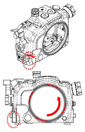
**STEP 2:** Carefully pull the port or extension ring out of the housing.
