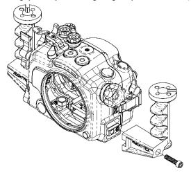
STEP 2: If you are adding any shoes, brackets or ball mounts onto your housing, mount them using the intended ½-20 UNC threaded holes. You can use the threaded holes on the handle grips (#1,#2), the top one (#3) or the bottom ones (#4) for
