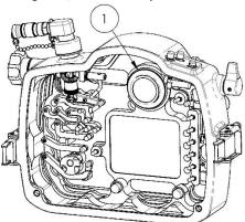
STEP 2: From inside the housing, slowly apply pressure to the viewfinder until it pops out from the back of the housing.
