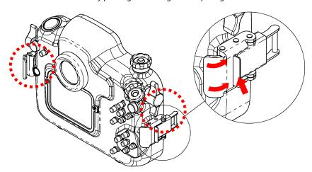
STEP 5: Pull the latches out so they don't interfere with the front section hooks upon closing.
