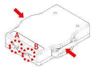
**WARNING:** Only use 2 x CR 2045-coin cell batteries to power your flash trigger. Using other types of batteries could cause damage to your flash trigger.
