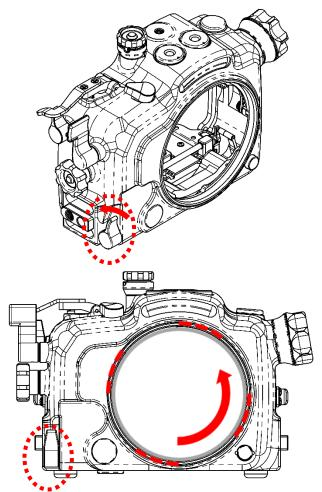
STEP 2: Carefully pull the port or extension ring out of the housing.
