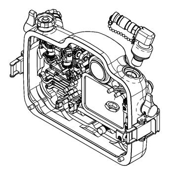
NOTE: Installation is shown on rear 1/2" bulkhead port.
