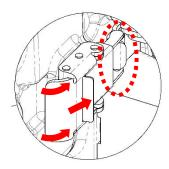
STEP 2: Rotate both latches to free them from the front hooks and pull out the rear section.
