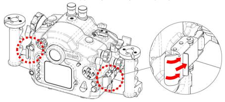
**STEP 2:** Rotate both latches to free them from the front hooks and pull out the rear portion.
