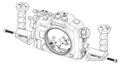
STEP 2: If you are adding any shoes, brackets or ball mounts onto your housing, mount them using the intended ¼-20 UNC threaded holes. You can use the threaded holes on the handle grips (#1,#2), the top one (#3) or the bottom ones (#4) for your tripod.
