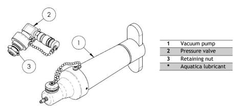
If your pump was not factory installed or bought separately, you will need to install the pressure valve bulkhead on your housing. You have two optional emplacements to install your vacuum pump system:
