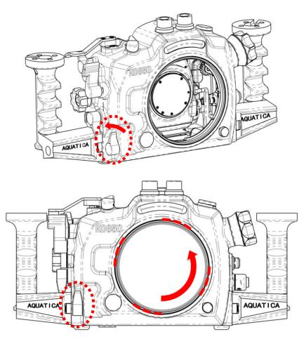
**STEP 2:** Carefully pull the port or extension ring out of the housing.
