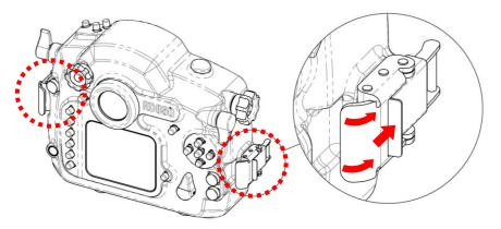
**STEP 5:** Pull the latches out so they don't interfere with the front portion hooks upon closing.
