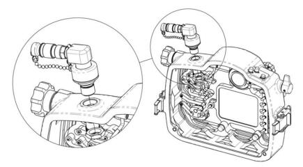
NOTE: Installation is shown on rear 1/2" bulkhead port.
